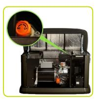
Note: Fuel pipe must be sized for full load. Required fuel pressure to generator fuel inlet at all load ranges 1.74-3.24 kPA (3.5-7" water column) for natural gas, 4.73-5.48 kPA (10-12" water column) for LP gas. Outputs are based upon values @ 1000 Btu per cubic feet with NG and 2500 Btu per
