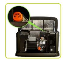
Note: Fuel pipe must be sized for full load. Required fuel pressure to generator fuel inlet at all load ranges 1.74-3.24 kPA (3.5-7" water column) for natural gas, 4.73-5.48 kPA (10-12" water column) for LP gas.
